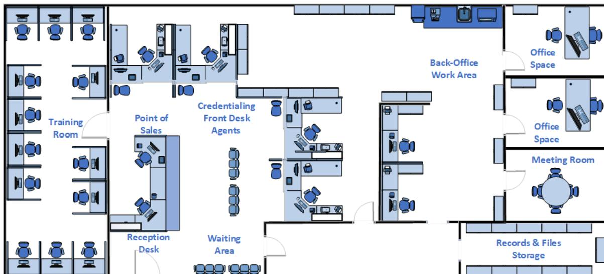
The small hub layout in Figure 2-3 is scaled down further, with more reduction in the number of back-office, front desk, and training positions, and a smaller waiting room area. The meeting room was removed, but a private office space is made available. Due to the smaller traffic volume, the receptionist position can be combined with the POS position.
