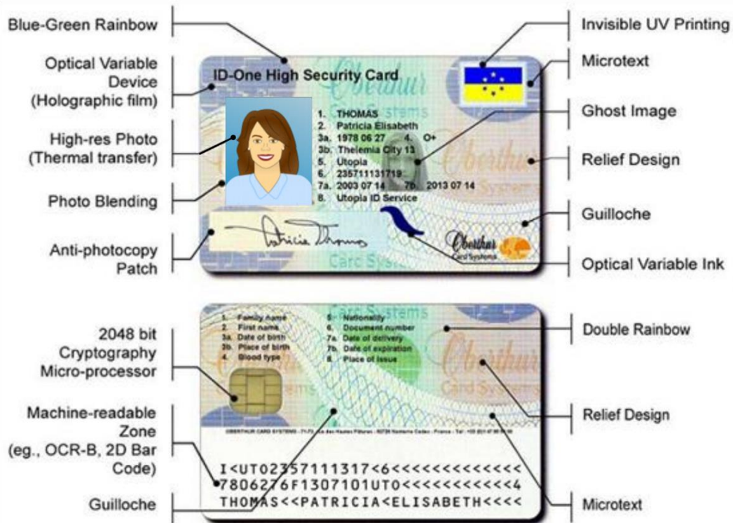
Figure 2-2. ACS Access Card with Enhanced Security Features
