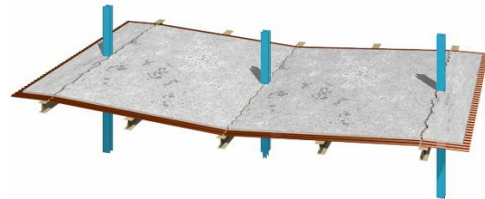
Figure B-13. Catenary Cable Floor Support System
