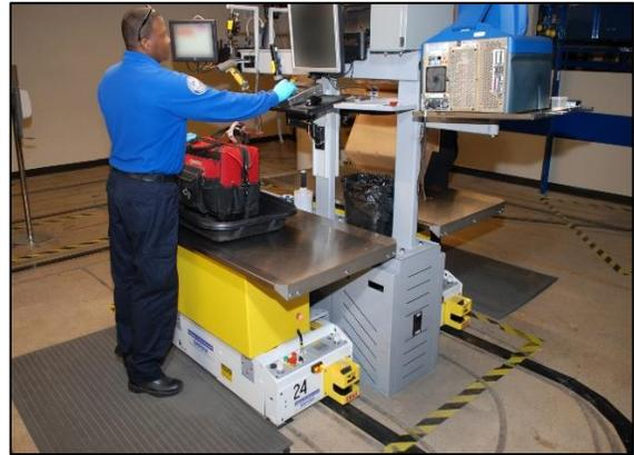
**Figure 3-3. Vanderlande FLEET Autonomous Checked Baggage Management System at DFW**
